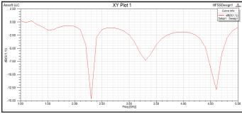
6. Return loss vs Frequency for Triangular Patch With DGS
