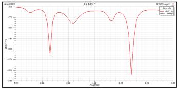
3. Return Loss vs Frequency for Circular Patch Without DGS
