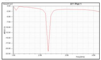
2. Return Loss vs Frequency for Rectangular Patch with DGS
