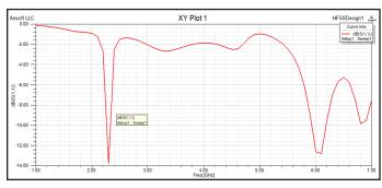
5. Return Loss Vs Frequency for Triangular Patch Without **DGS**
