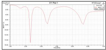
4. Return loss vs Frequency for Circular Patch with DGS
