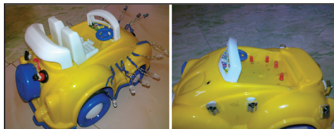
Fig. 8: The Transmitter (Left) and Receiver (Right) implemented on a toy car model. Here when the switch (Horn) is pressed on the transmitter car the infrared signals are transmitted to the second car and the sound is produced in appropriate direction (here apart from buzzers, LED's are used to indicate the direction).
