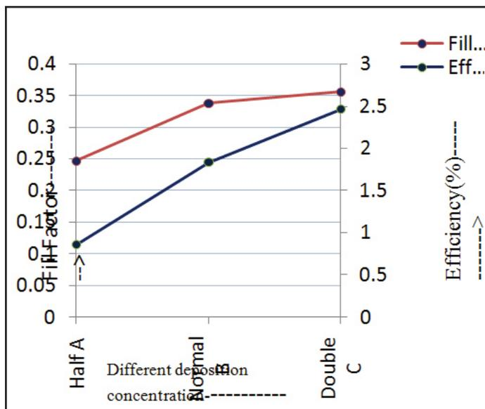
Fig. 6: Variation of Fill Factor and Efficiency With Different Concentration of Precursor Solution of Photo Electrodes
