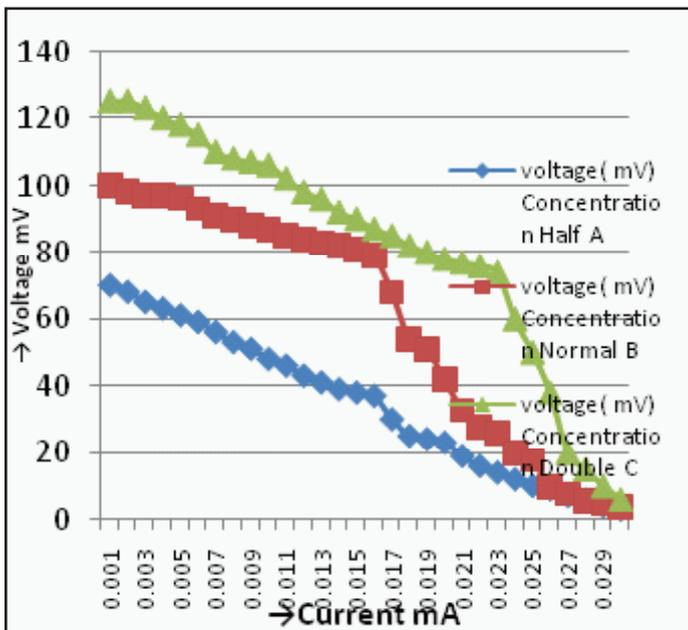
Fig. 4: I-V Characteristics of PEC Solar Cells for Photo Electrodes Prepared for Different Concentration of Precursor Solution
