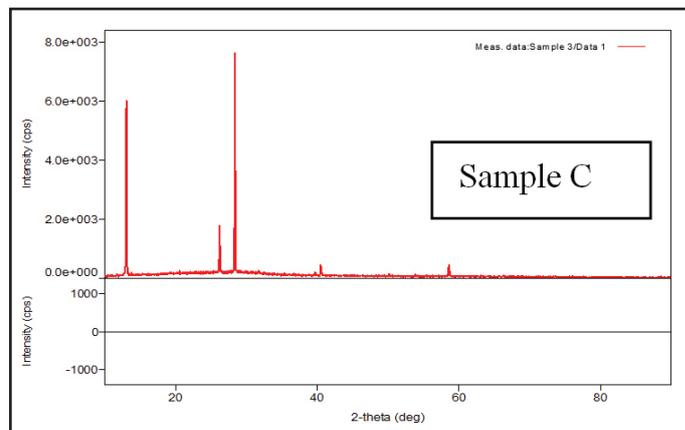
Fig. 2: [A][B] [C] X-ray Diffraction Pattern of Deposited CdTe thin film for half concentration A, normal concentration B, double concentration C of precursor solution respectively.
