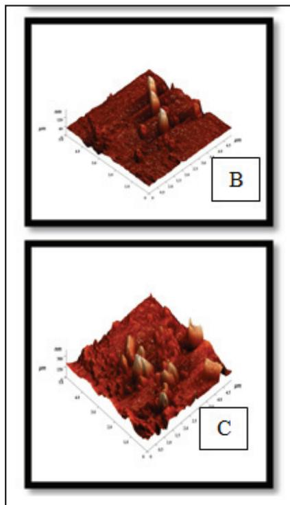
Fig. 3: [A], [B], [C] shows AFM 3D image confirming surface morphology of CdTe thin film for half A, normal B and Double C Concentration of Precursor Solution Respectively.
