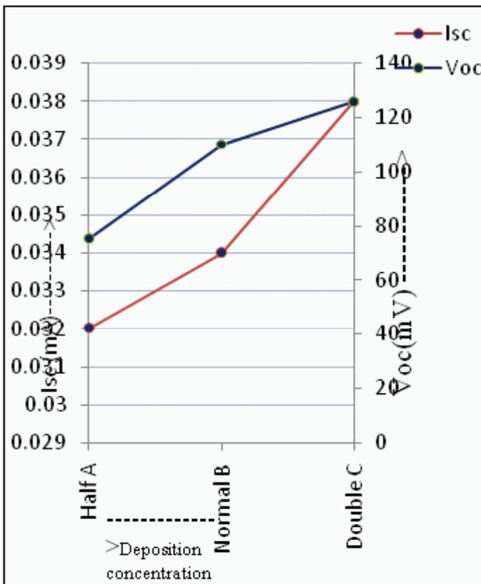
Fig. 5: Variation of  $V_{oc}$  and  $I_{sc}$  With Different Deposition Time of Photo Electrodes
