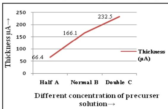
Fig. 1: Thickness of the Films as a Function of Concentration of Precursor Solution
