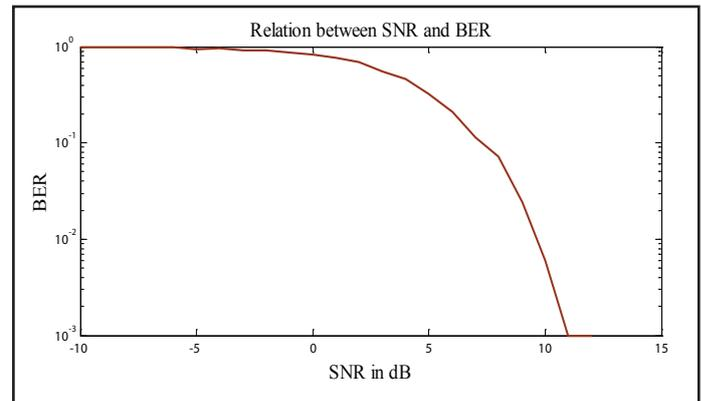
Fig. 1: Relation Between SNR and BER in TD-CDMA System
