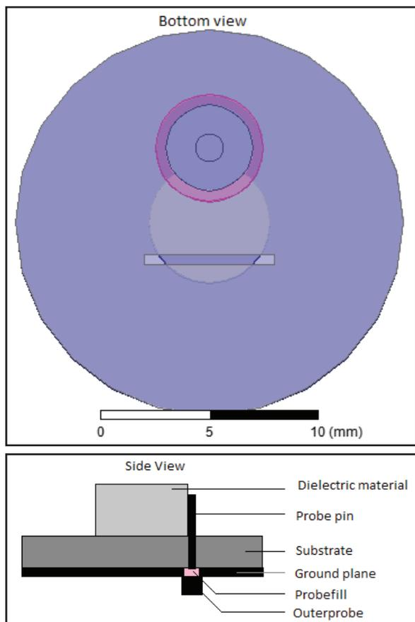
Fig. 1(a): The Top View of CDRA, (b) Bottom view of CDRA (ground plane).
