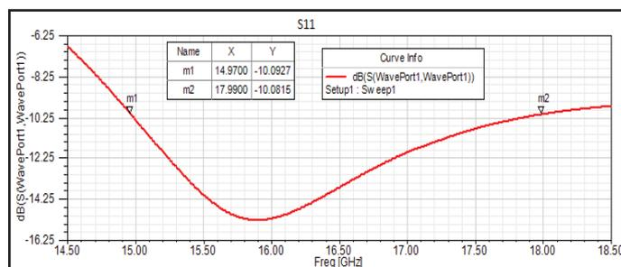
Fig. 2: Simulated Return Loss Versus Frequency
