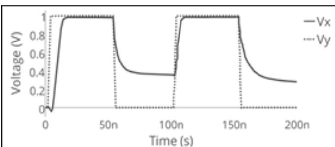
Fig. 8: Transient Analysis verifying  $V_x = V_y$
