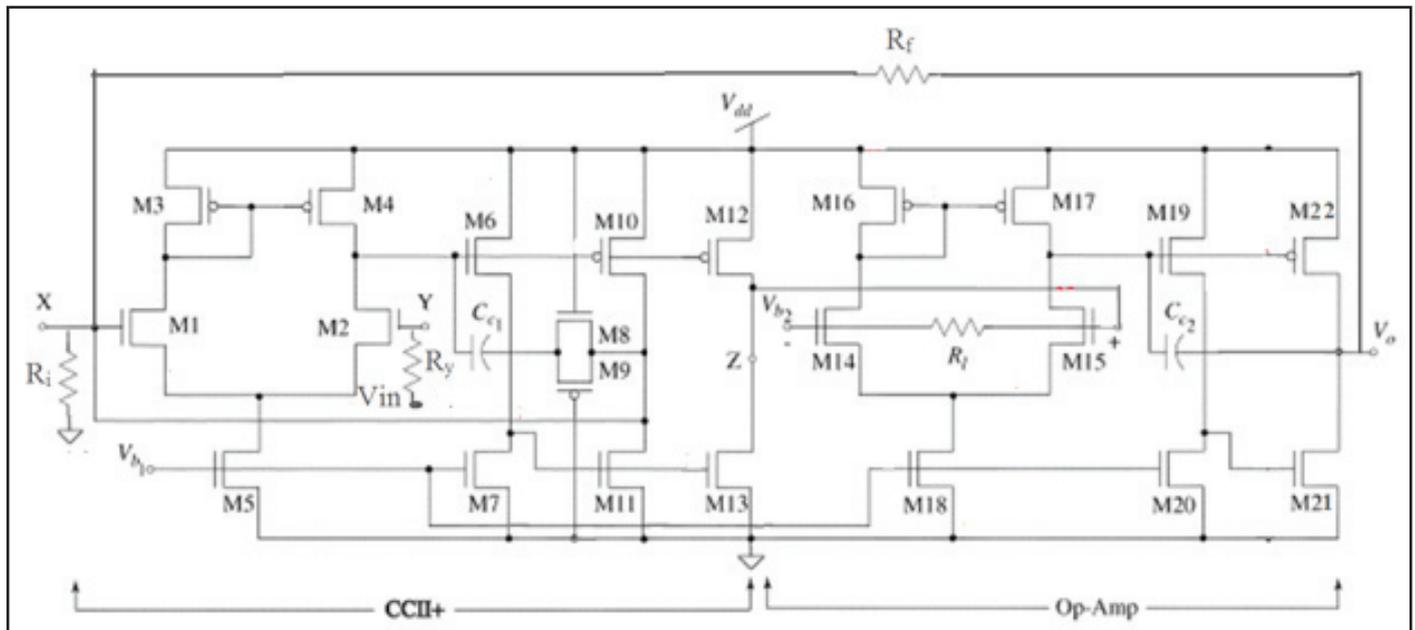
Fig. 4: Circuit diagram of proposed CFOA
