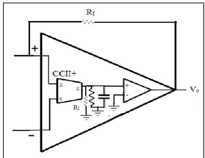
Fig. 3: CFOA made using CCII+ and opamp
