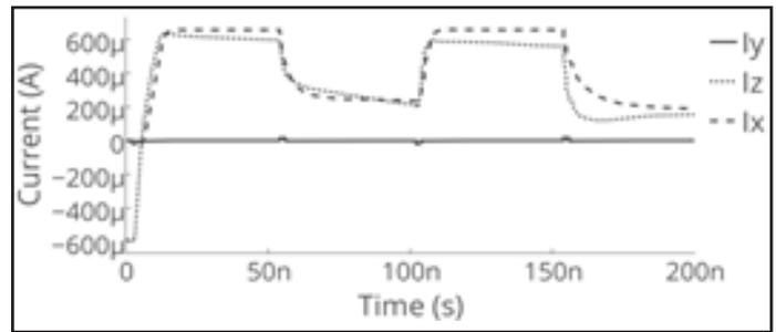
Fig. 9: Transient Analysis verifying  $I_x = I_z$  and  $I_y = 0$
