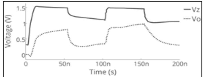
Fig. 10: Transient Analysis verifying  $V_z = V_o$
