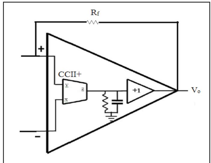
Fig. 2: Conventional CFOA made using CCII+ and voltage buffer
