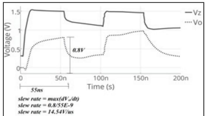
Fig. 11: Calculation of slew rate from output transient graph
