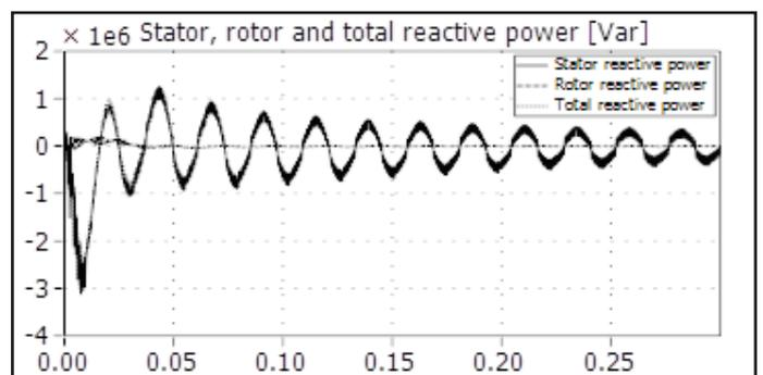
Fig. 11: Stator, Rotor and Total Active and Reactive Power
