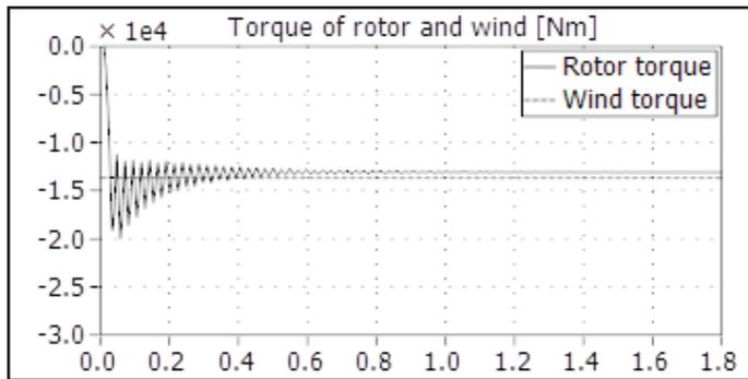
Fig. 12: Mechanical Oscillations at Startup of the Wind Turbine
