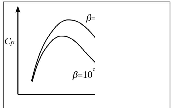
Fig. 2: Typical Performance Coefficient Vs. Tip Speed Ratio Curve
