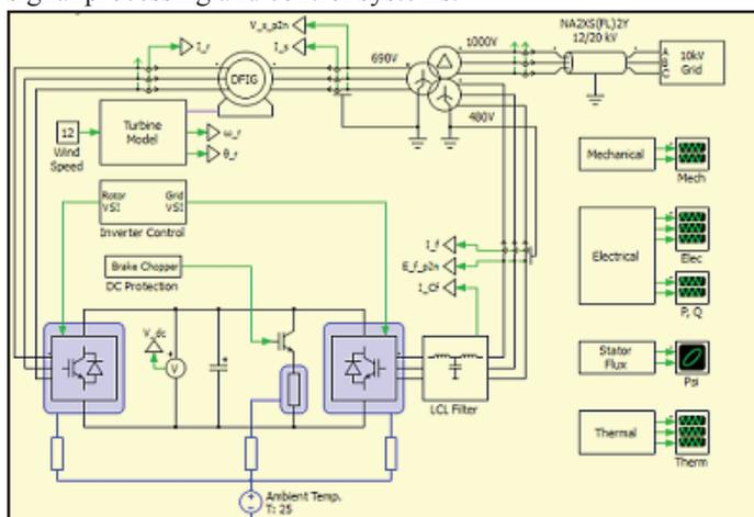
Fig. 3: Schematic of the DFIG Wind Turbine Model in PLECS
