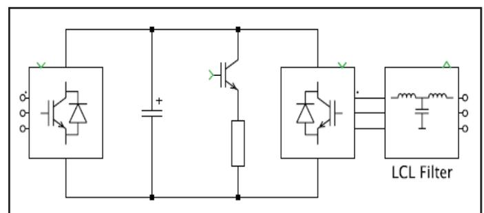
Fig. 5: Back-to-Back Converter Model
