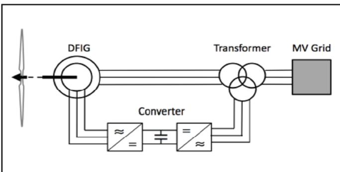
Fig. 1: System Overview of the Wind Turbine With DFIG
