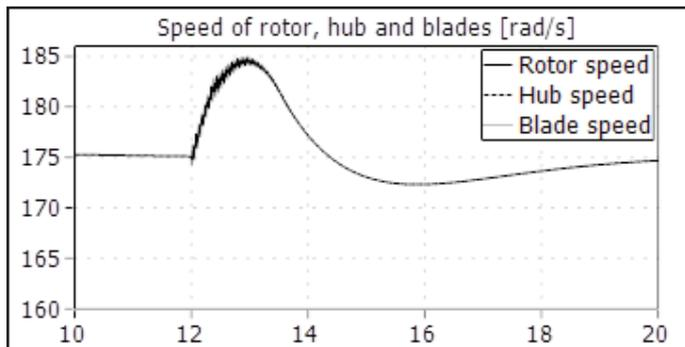
Fig. 13: Mechanical Transient During Grid Fault
