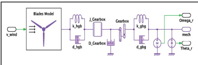
Fig. 6: Complete Drivetrain Modeled in the PLECS Mechanical Domain
