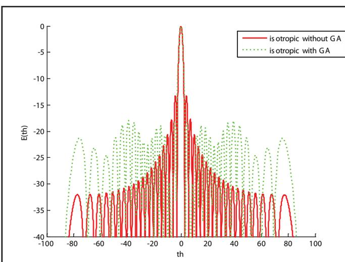
Fig. 4: Radiation Pattern of Isotropic Array for N=20 Elements
