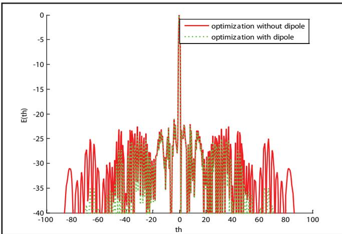
Fig. 3: Radiation Pattern of Thinned Array for N=60 Elements
