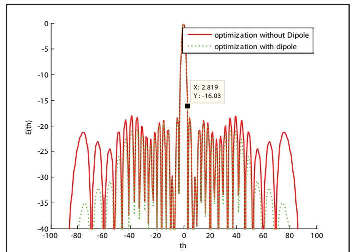
Fig 1: Radiation pattern of thinned array for N=20 elements
