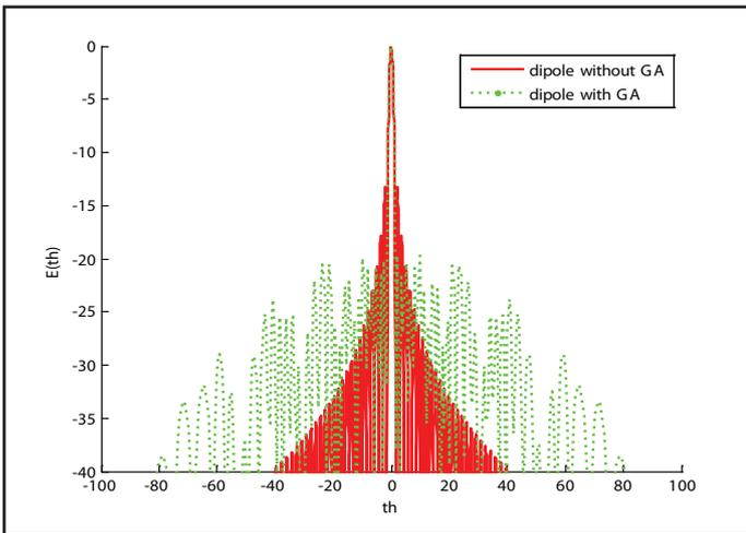
Fig. 8: Radiation Pattern of Dipole Array for N=40 Elements
