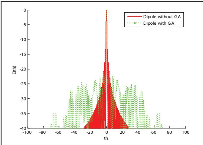
Fig. 9: Radiation Pattern of Dipole Array for N=60 Elements
