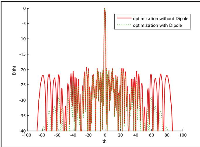
Fig. 2: Radiation Pattern of Thinned Array for N=40 Elements
