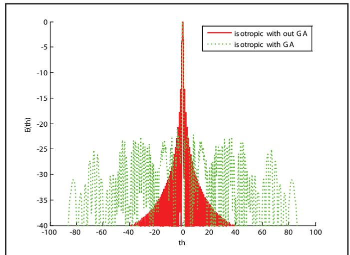
Fig. 6: Radiation Pattern of Isotropic Array for N=60 Elements
