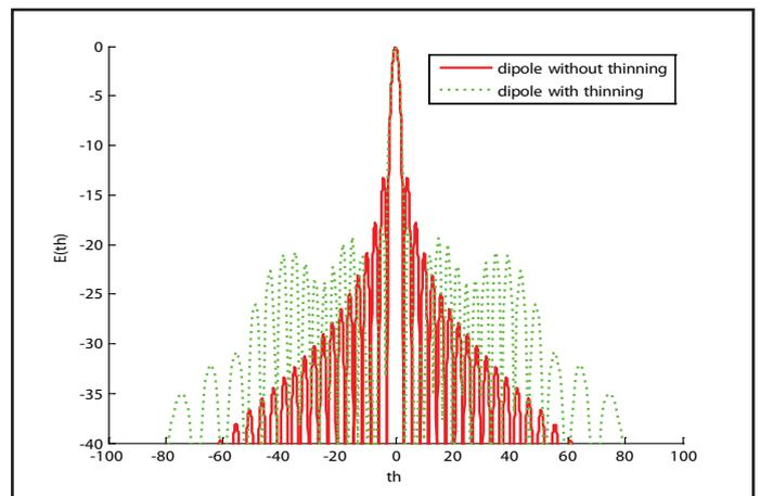
Fig. 7: Radiation pattern of Dipole array for N=20 elements
