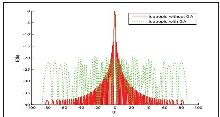
Fig. 5: Radiation Pattern of Isotropic Array for N=40 Elements
