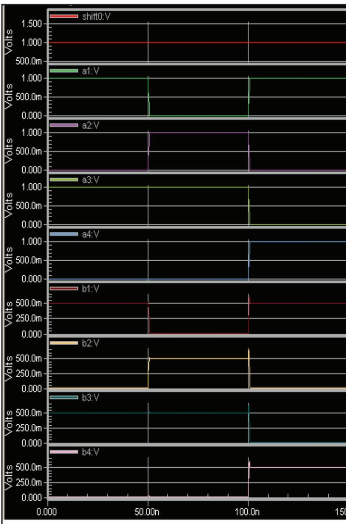
From the above graph is only for Shift-0, where the input output connections are same as truth table like  $a_1-b_1, a_2-b_2, a_3-b_3, a_4-b_4$ .
