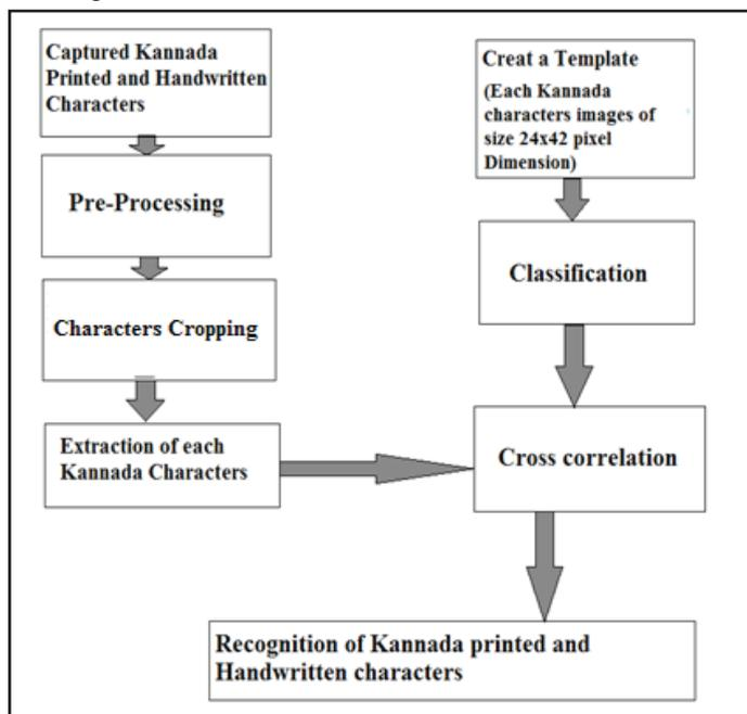
Fig. 1: A Block Diagram of the Proposed Algorithm
