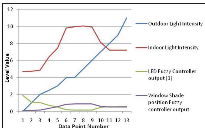
Fig. 3.1: Line Graph for Effect of Outdoor Light Intensity
