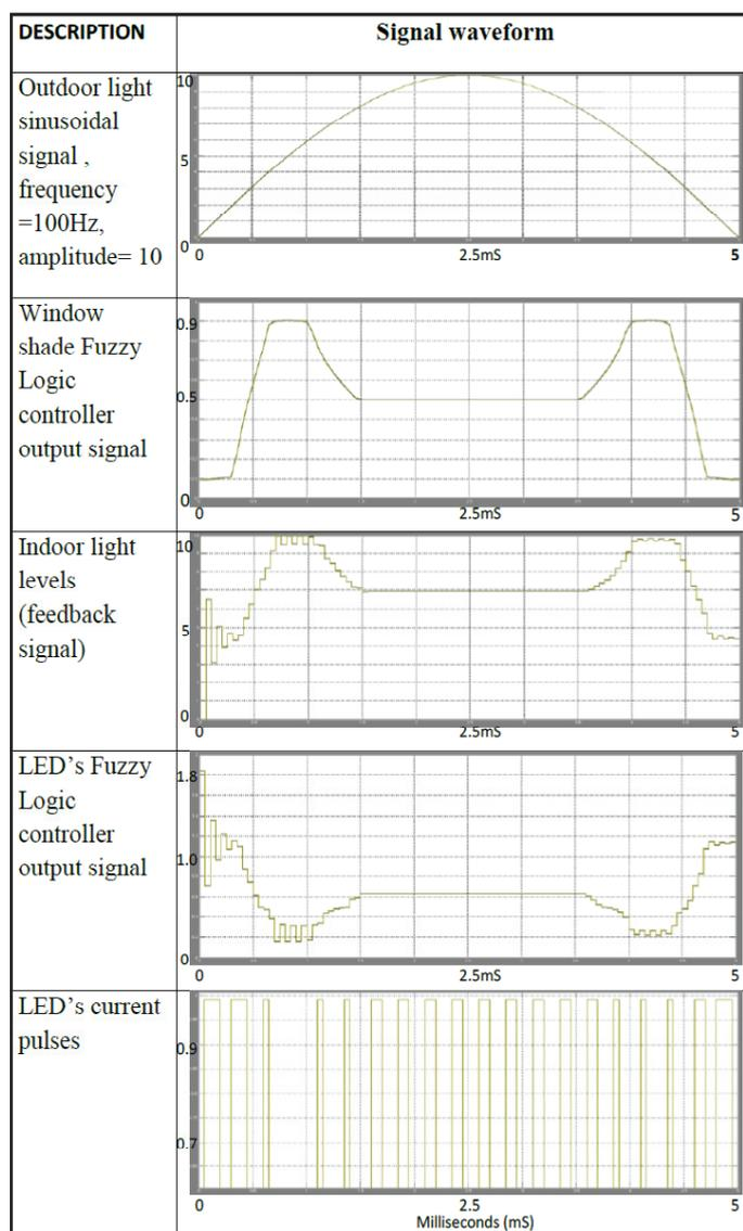
Fig. 3.2: Signal Waveforms Incorporating the Effect of Outdoor Light
