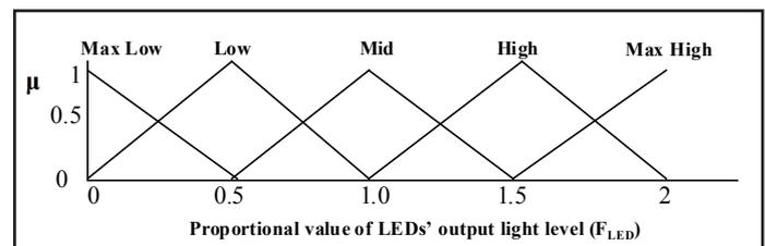
Fig. 2.10: LEDs’ light – Output Membership Function
