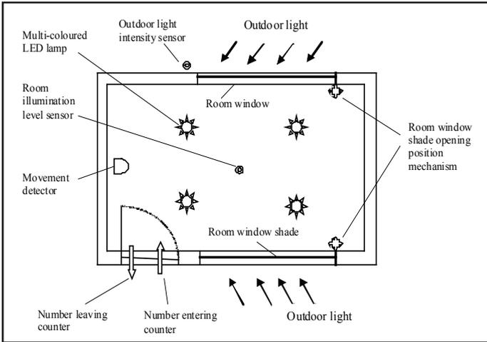
Fig. 2.4: Typical Room Diagram With Controlled Light
