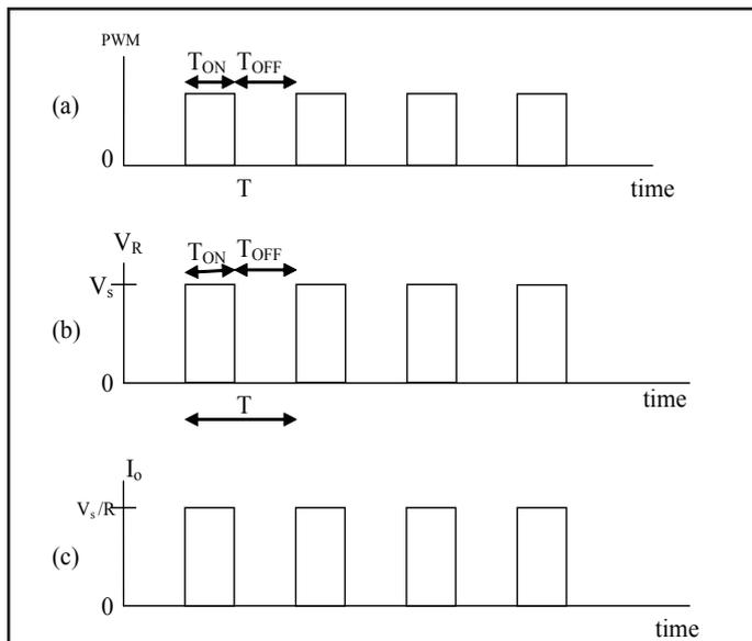
Fig. 2.2: Theoretical Waveforms for the Driver Pulses
