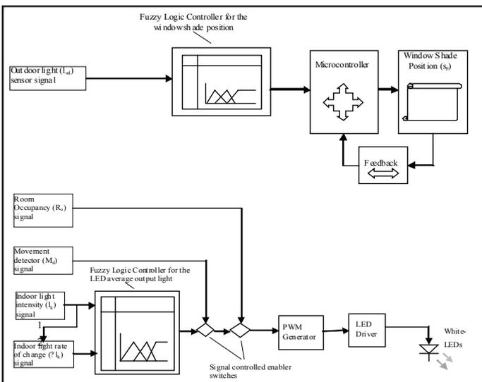
Fig. 2.5: Basic Scheme for the Room Lighting Control
