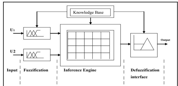
Fig. 2.3: Illustration Diagram for Fuzzy Logic Controller
