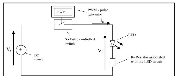
Fig. 2.1: Circuit Diagram PWM Controlled LED Driver
