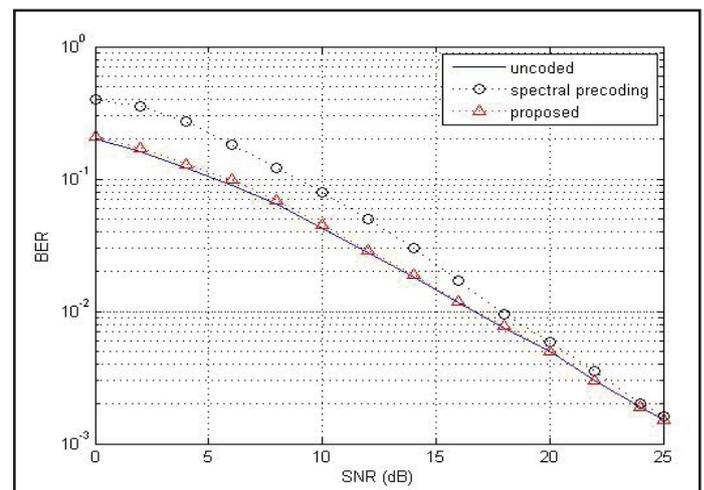
Fig. 8: BER Performance Comparison of the Proposed and Existing Systems
