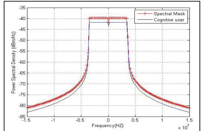
Fig. 7: Proposed Spectral Mask Without Using Notch Frequencies
