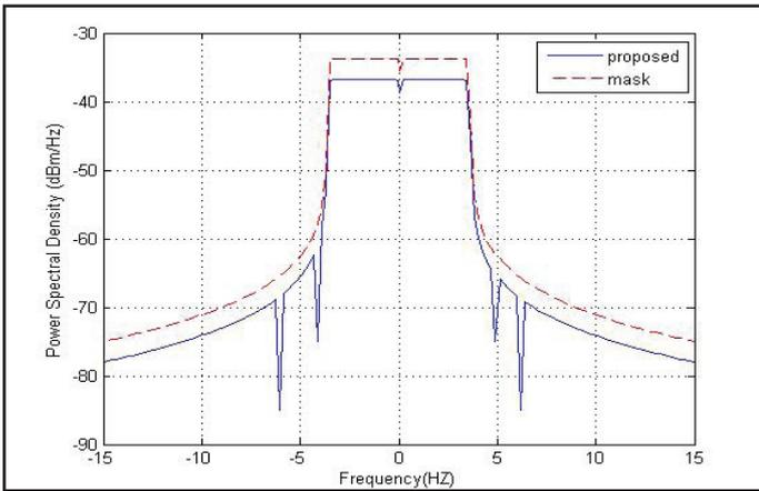
Fig. 4: Spectral Precoding Using Notch Frequency Technique
