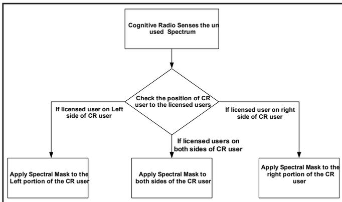
Fig. 3: Block Diagram of Efficient Utilization of Spectral Mask Techniques
