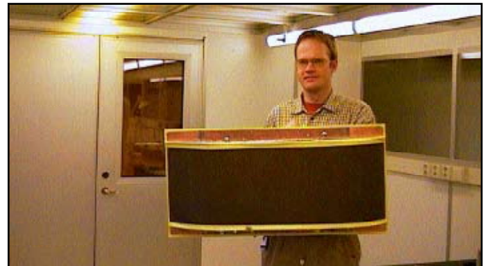
Fig. 10: Picture of an 8-Element Array Antenna at 1.8 GHz. (Antenna Property of Telia Research AB, Sweden)
