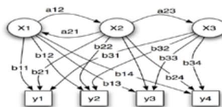
Fig.1. State Transition in HMM: x - hidden states, y - observable outputs, a - transition probabilities, b - output probabilities plays an important role in this context, and depends strongly on the precise acoustic modeling of speech. Some of the most important applications of digital signal processing techniques have been in the area of speech processing. In fact, a large percentage of the theoretical 'background or digital signal
